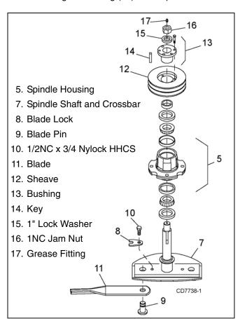
Figure 15. Sheave and Blade Assembly
